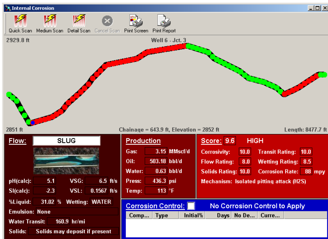
Fig. 12: The Internal Corrosion Screen, Showing a Detail Scan of a Pipeline with a High Corrosion Risk Assessment.
